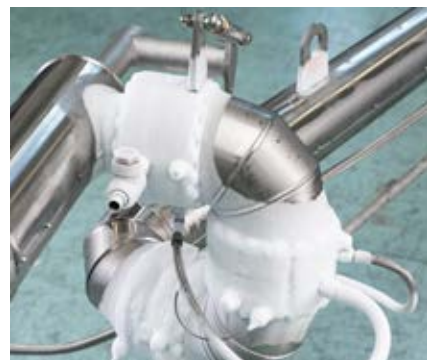
Cryoload swivels under load during FAT
