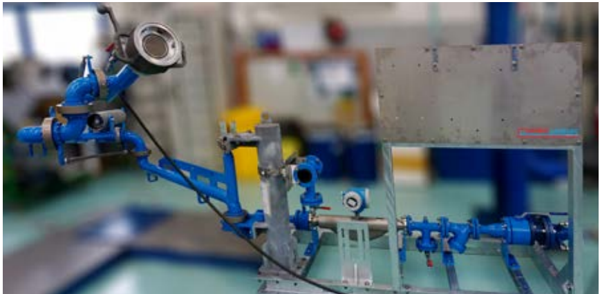
Bottom loading skid with meter, filter and controller - UK - Renewable Fuels industry
