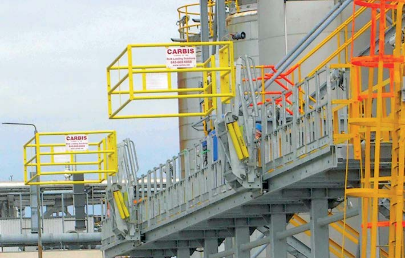
2 x Tracking Gangways (Folding Stair) with 20m track and swing shut gates - UK - Chemical industry
