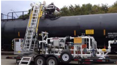
Transloading skid used to transfer product from rail cars direct to road tankers with no intermediate storage facility
